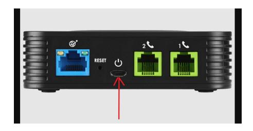
**Step 1:** Locate the power cable. It will be plugged into the port indicated (red arrow).
